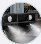
Spray Water To Reduce Dust
