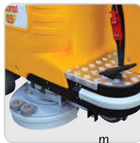
Strong brushes base with independent reduction gears.
